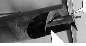
Wrap flighting in behind original up to gusset and weld together.
